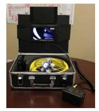
Rainbow MWD recently incorporated new technology in our water mainline inspections during emergency and scheduled repairs. With the use of this camera equipment, pictured to the right, we are able to inspect the internal coating inside the water mains during water main shutdowns.
