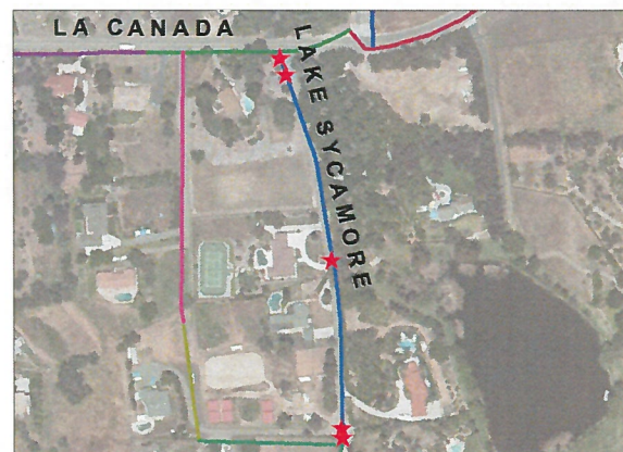
District break data suggests that a 930' project on Lake Sycamore Drive may have a CML construction quality issue at the joints.
